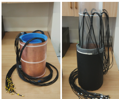
Figure 4. Pictures of two experimental constructions of 3D ECT sensors under study.
