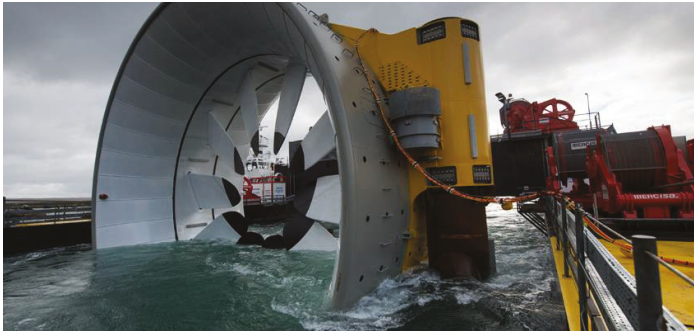
Figure 1. OpenHydro/Naval Energies direct-drive tidal stream turbine [4].
