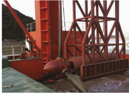
Figure 3. Small scale multibrid tidal stream turbine [15].
