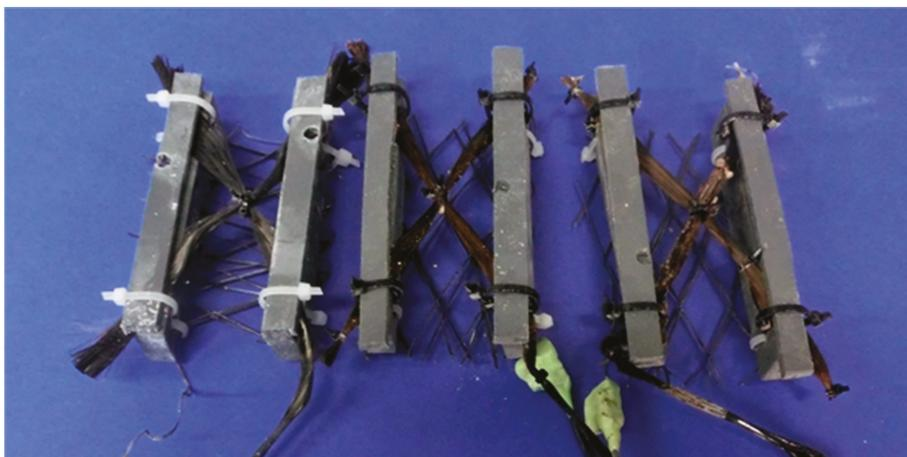
**Figure 11.** From left to right: specimen P1 of levels 1 to 3 after polarization.
