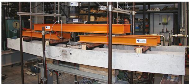
**Figure 5.** Test setup of the carbon concrete girder.
