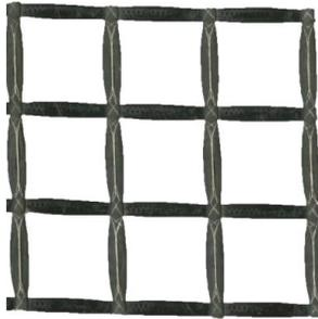
Figure 1. Carbon textile impregnated with epoxy resin.
