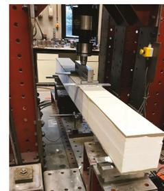
Figure 6. Four-point bending test set-up.
