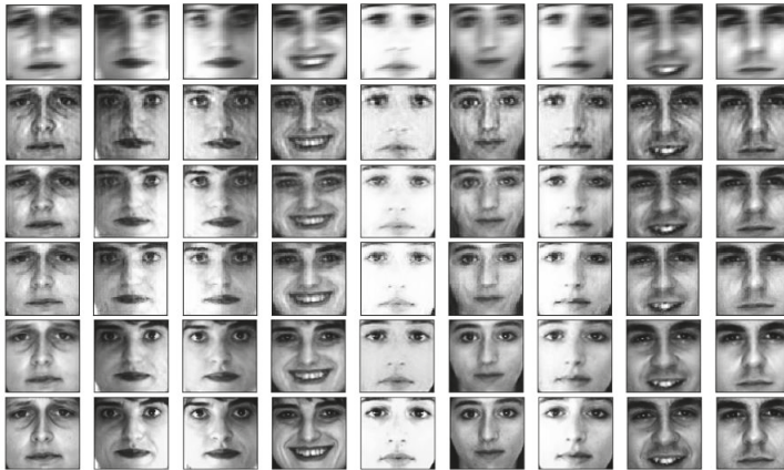
Figure 3. Restored images of human face. The first row shows the images with motion blur; the images from the second row to the fifth row are restored images of DnCNN, ResNet, ResNet with dilated convolution and FbResNet; the last row shows the clean images.
