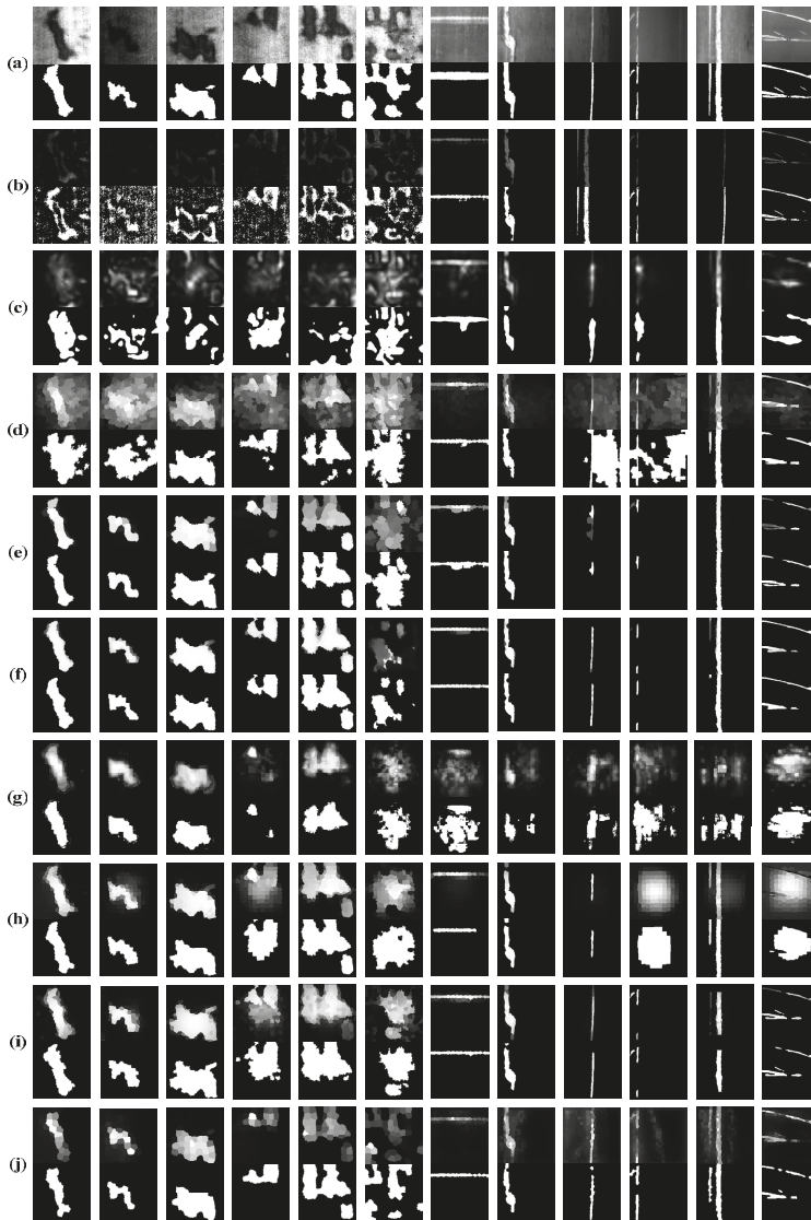
Figure 5. Qualitative comparisons: (a) ground-truth; (b) RPCA; (c) IS; (d) ULR; (e) RBD; (f) SBD; (g) DSR; (h) RS; (i) SMF; (j) Ours. We can see that our segmentation results, which are produced by simple Otsu’s method on the saliency map, are very closer to the ground truth.
