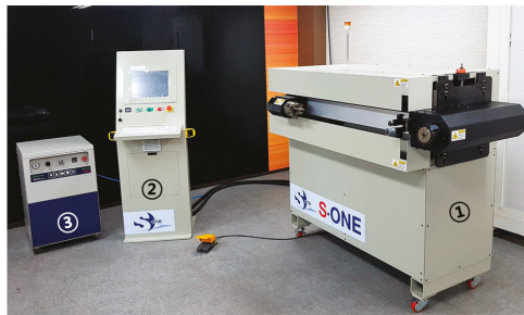
Figure 6. Establishment of CNC bending machine. In the figure, components of the CNC bending machine are (1) main body, (2) control cabinet, and (3) air pump.
