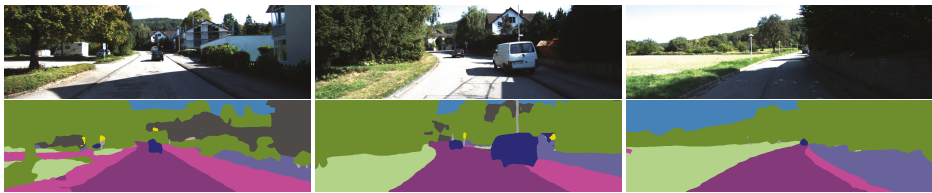
Figure 6. Instances of 2D semantic segmentation in the KITTI odometry set.
