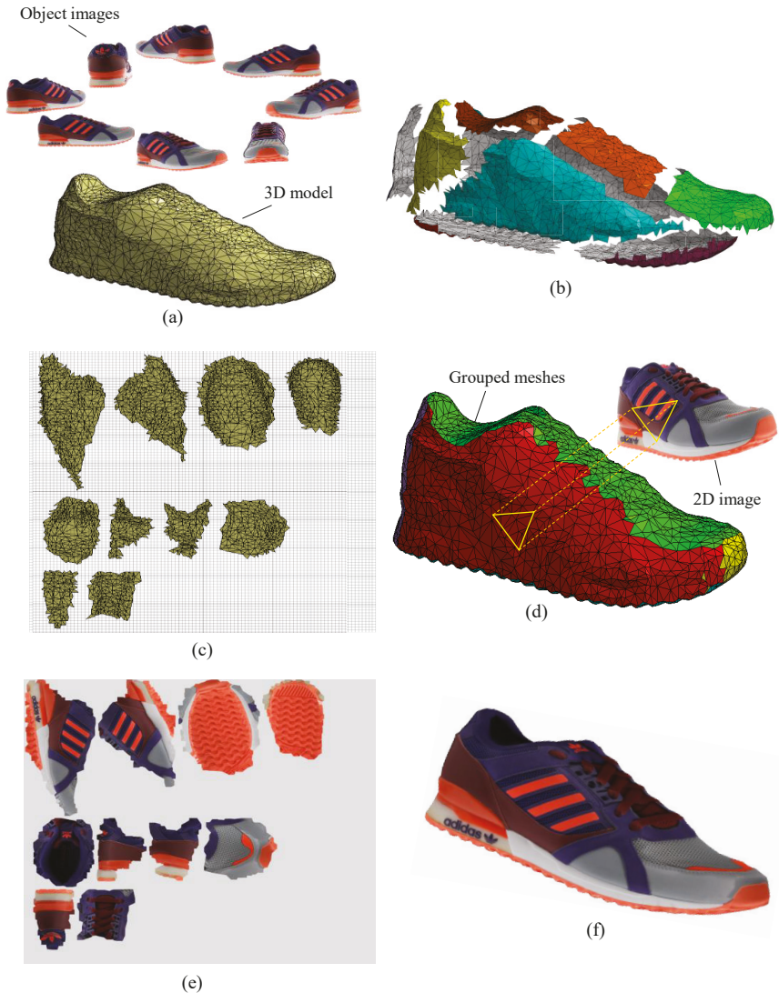
Figure 1. Overall flowchart of the proposed texture mapping method: (a) input data, (b) mesh partitioning, (c) mesh parameterization and packing, (d) texture transferring, (e) correction and optimization, and (f) output object file.
