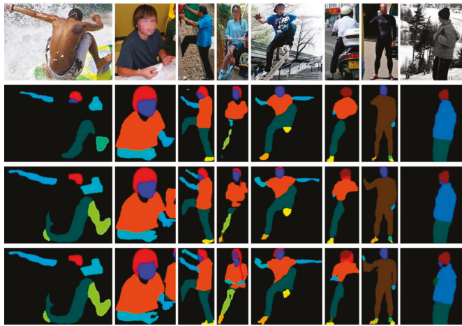
Figure 8. Performance comparison between the OM and the SM on the validation set. From the top row to the bottom row are input images, predictions from the SM, predictions from the OM and the ground truth labels.
