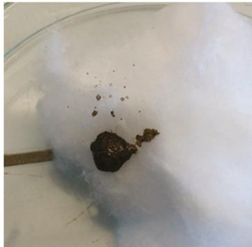
**Figure 9.** Photograph showing the formation of black residue at the surface of cotton after the UL-94 test.
