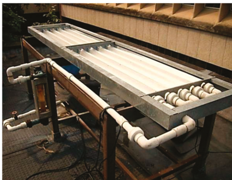
Figure 8. Solar pilot-scale CPC reactor (Photocatalysis lab, Universidad del Valle, Cali, Colombia).
