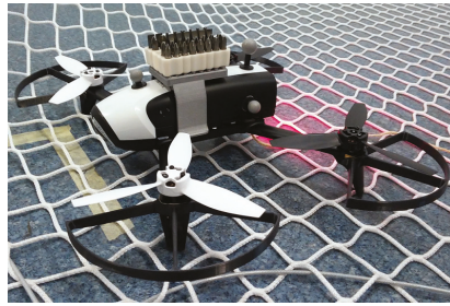
Figure 18. The Bebop 2 with additional payload used for in-flight auto-tuning experiments.
