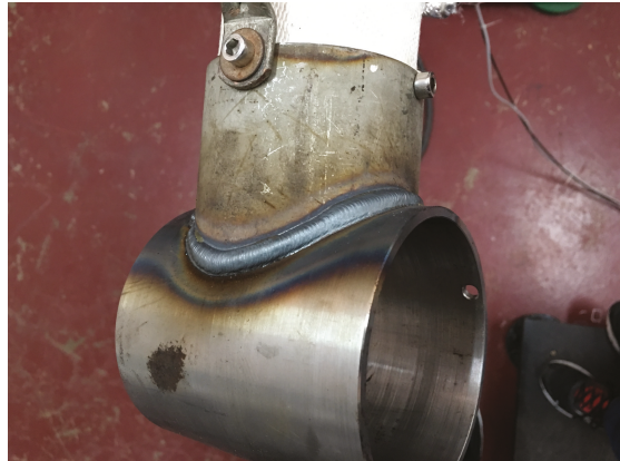
Figure 21. Pipe-connect-pipe arc welding result.
