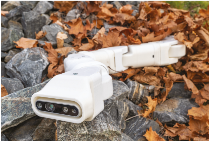
Figure 1. Serpens : A low-cost ROS-based snake robot with series elastic actuator (SEA), precision torque control and a screw-less assembly mechanism.
