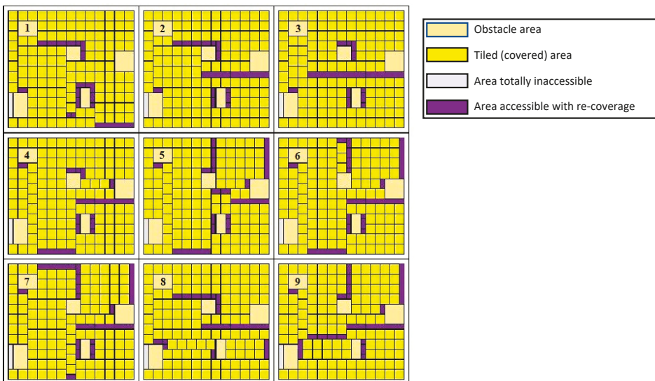
Figure 14. Sample sweeping solutions with fixed morphology and no tiling theory.
