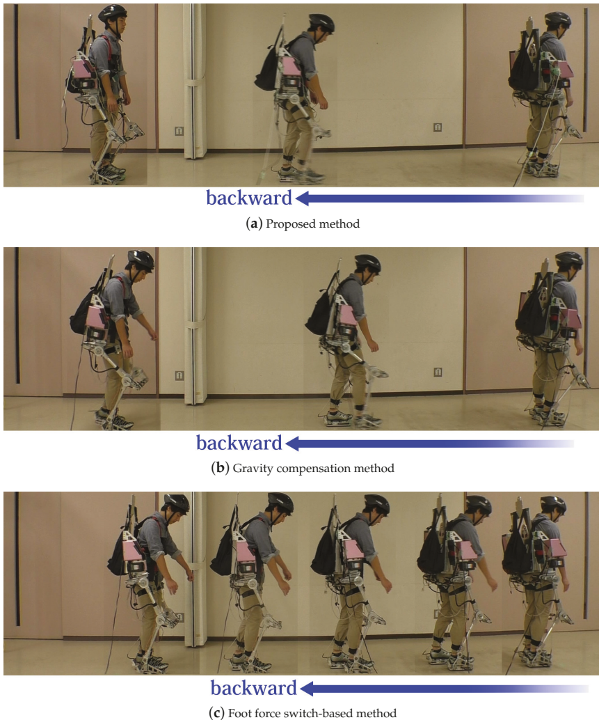
Figure 9. Image sequences of walking backward based on each method: the sampling time of the image capture was approximately 5.4 s.
