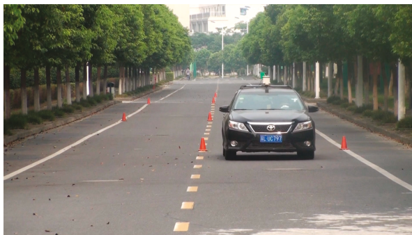
Figure 2. Single lane change test.
