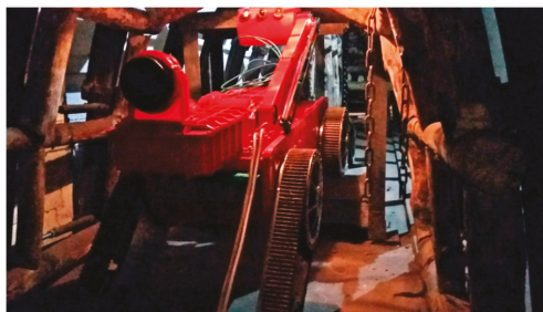
Figure 15. TeleRescuer—testing in a training coal mine Queen Luiza (March 2018).
