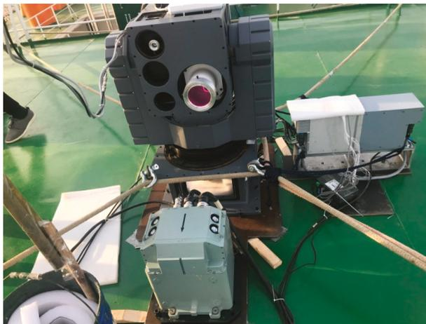
**Figure 6.** The shipborne ATP system. The shipborne ATP system shows the uplink beacon, coarse camera, and the attitude pre-compensation unit.
