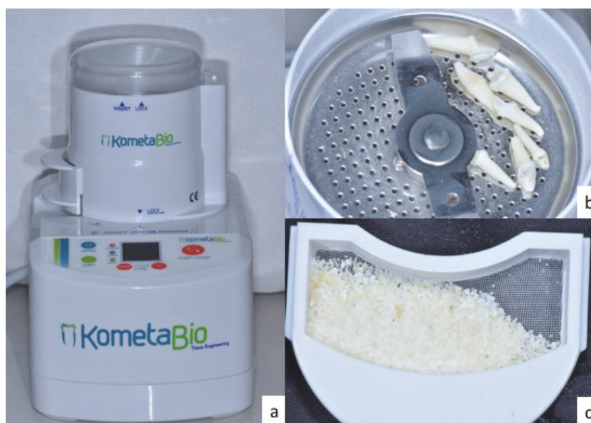
Figure 2. (a) Smart dentin grinder device; (b) Dog's extracted premolar teeth inside grinding chamber; (c) Tooth particles of 300–1200 microns obtained after using the grinding device.
