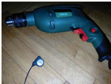
Figure 7. Capacity microphone (ZALMAN ZM-MIC1 microphone) and the commutator motor (electric impact drill).
