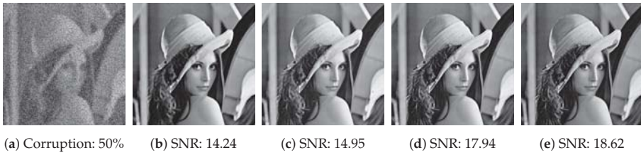
Figure 13. Comparisons of TVL1, HTVL1, CTVL1 and HOCTVL1 model on the Lena image corrupted by Gaussian blur and random-valued noise with noise level 50%. (a) Corrupted image. (b) TVL1 model. (c) HTVL1 model. (d) CTVL1 model. (e) HOCTVL1 model.
