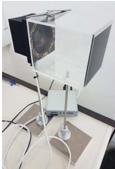
Figure 6. The three ways to use the suggested sensor and its associated recorder: by tethering an insect inside the probe volume of the sensor (e.g., by holding its legs with an inverted tweezer), by confining the insect in a transparent cage that is large enough to allow the insect to fly, or by inserting the sensor in an insectary cage containing a free-flying insect. Notice the black termination plane on the right of the Plexiglas (MAXiBLACK, Advanced Coating Products, Acktar Store LTD, Kiryat-Gat, Israel).
