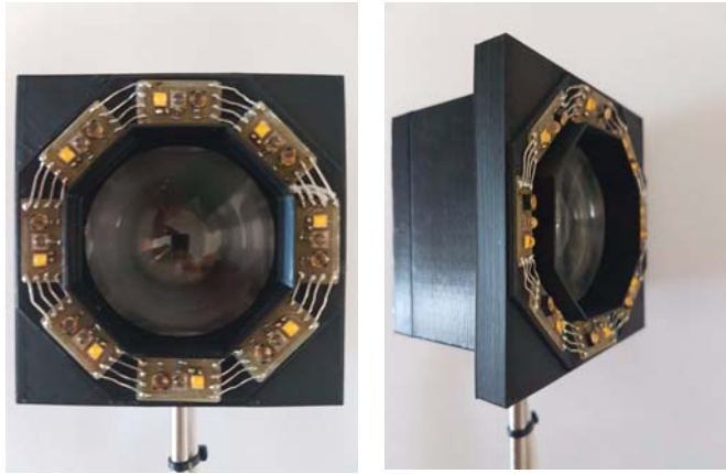
Figure 1. The multispectral sensor: (left) The disk in the middle is the Fresnel lens. The three LED's in each plate emit, in turn, visible light 450–700nm, and infrared at 810 nm and 940 nm. All eight LEDs of each spectral band are lit simultaneously for 20.8 microseconds (i.e., three circular arrays of eight LEDs each). All LEDs' supporting plates have a 68.5° orientation with respect to the Fresnel plane (right). The photodiode is placed at the focal point of the Fresnel lens.
