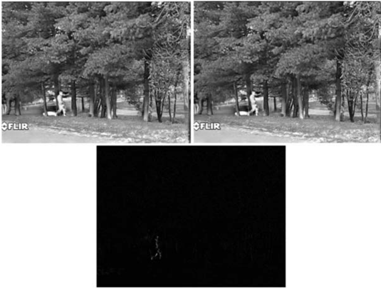
Figure 7. Fused two successive frames (top images) and difference image obtained between these two frames (bottom image).
