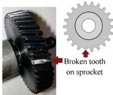
Figure 3. Broken tooth on sprocket of the electric impact drill.
