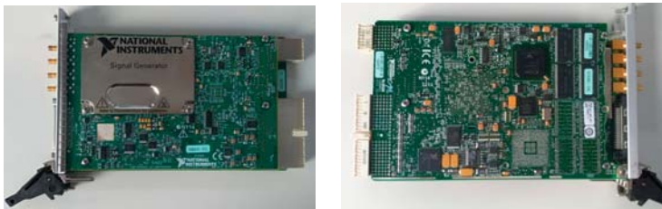
Figure 12. Hardware architecture of arbitrary waveform and signal generator.
