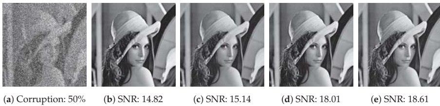
Figure 9. Comparisons of TVL1, HTVL1, CTVL1 and HOCTVL1 model on the Lena image corrupted by Gaussian blur and salt-and-pepper noise with noise level 50%. (a) Corrupted image. (b) TVL1 model. (c) HTVL1 model. (d) CTVL1 model. (e) HOCTVL1 model.
