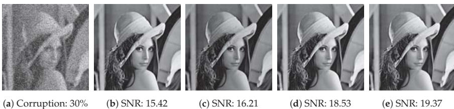
Figure 8. Comparisons of TVL1, HTVL1, CTVL1 and HOCTVL1 model on the Lena image corrupted by Gaussian blur and salt-and-pepper noise with noise level 30%. (a) Corrupted image. (b) TVL1 model. (c) HTVL1 model. (d) CTVL1 model. (e) HOCTVL1 model.
