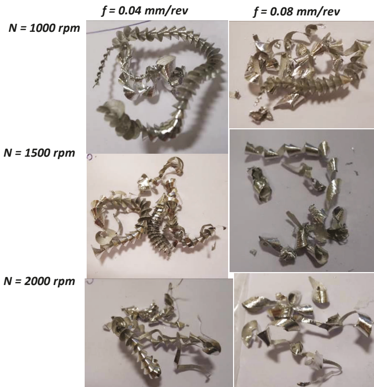
Figure 11. Cutting chips after drilling of 10th hole at different spindle speed and feedrate.
