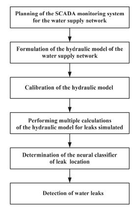
Figure 1. Block diagram of the algorithm for detection and location of hidden leaks.
