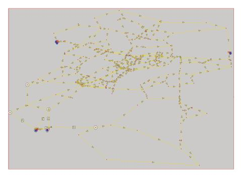
Figure 2. The modelled water network; ZB on the network graph means tank and SP means pumps station.
