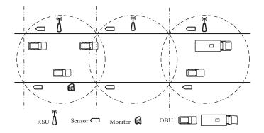
Figure 1. Application scenarios under the Polling Control with Sleeping media access control (PC-S MAC) protocol. OBU: on-board unit; RSU: roadside unit.
