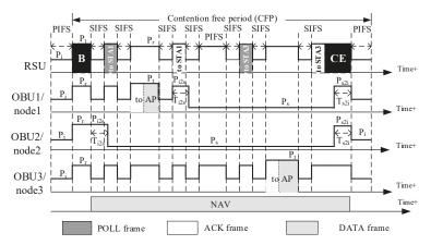
**Figure 2.** PC-S MAC: Active OBU1/node1 and OBU3/node3 transmit safety and traffic data packets to the RSU in order, while OBU2/node2 in idle state turns into sleep after receiving the beacon and downlink data from the RSU. CE: CFP\_END ; STA: station; PIFS: point interframe space; SIFS: short interframe space.
