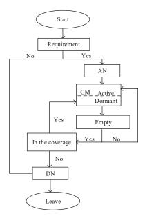
Figure 3. State transition diagram of the PC-S MAC. AN: Applicant Node; CM: Cluster Member; DN: Dissociative Node.
