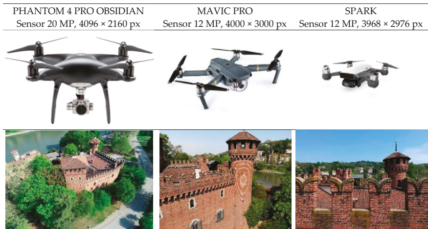
Figure 5. Different Unmanned Aerial Vehicle (UAV) platforms by DJI company and related sensors with captured images.
