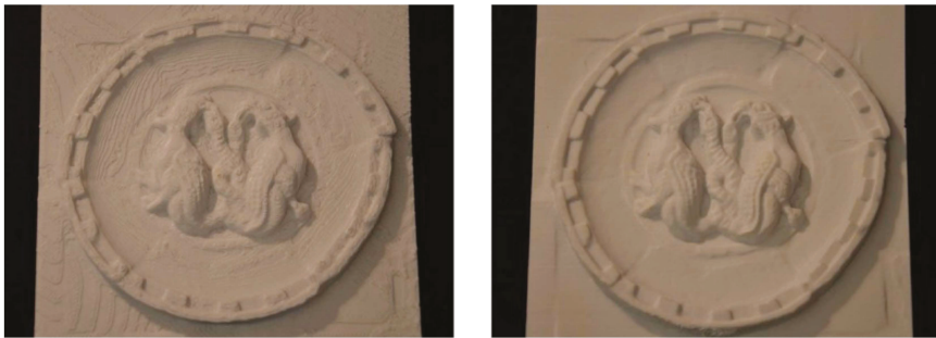
Figure 2. Different quality of replica due to the slicing orientation of the model on the printing plate. (left) Longitudinally with evident traces of layers; (right) diagonally, without traces of layers.
