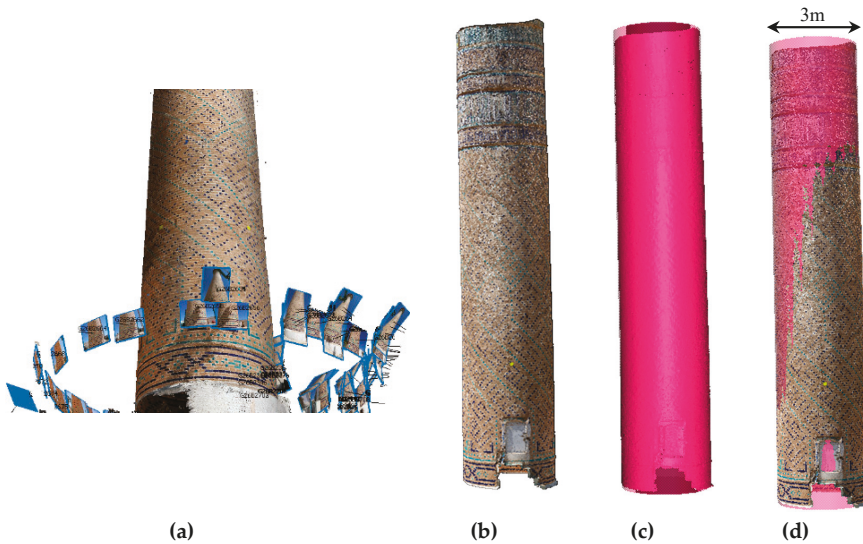
Figure 9. The produced image-based point cloud of the shrine minaret. (a) Minaret body with the oriented images around it. (b) Dense point cloud of the minaret. (c) Best fitting cylinder. (d) Fitting cylinder fused with the point cloud.
