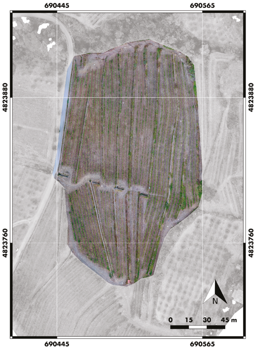
Figure 4. The orthophoto of the study area produced by the photogrammetric processing of the images acquired from the RGB flight over the Grospoli vineyard.
