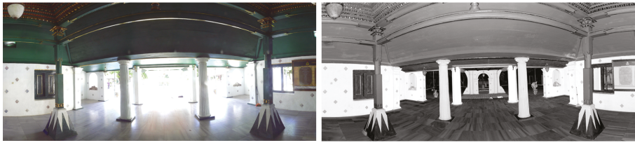
Figure 3. Example of a section of a panoramic image captured by the TLS. The figure to the left shows the RGB image, with strong overexposure due to sunray intensity. The figure to the right shows the intensity image, which was preferred in the tie point identification process.
