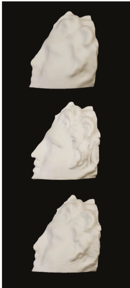
Figure 13. The three printed replicas: from above, first photogrammetry, laser-scanning, and second photogrammetry.
