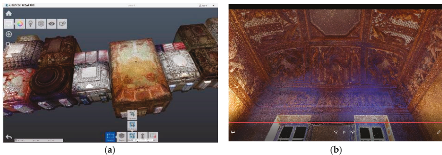
Figure 22. (a) A screenshot of the LiDAR points model managed in the Recap environment; (b) A screenshot from the video navigation achieved from LiDAR points cloud.
