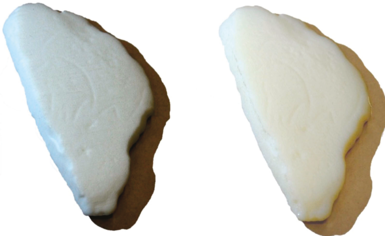
Figure 4. (left) Replica in Nylon PA 12; (right) replica in glass-filled nylon.
