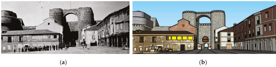
Figure 10. Extramural buildings: (a) old photograph texture integration (Laurent, c. 1865, Ruiz Vernacci Archive, VN-17214); (b) with 4D modeling for the extramural section of the Alcázar gate. Source: Cultural Heritage Institute of Spain (IPCE). [1].
