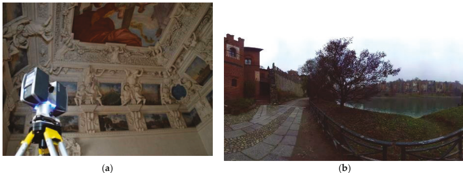
Figure 3. Terrestrial Laser Scanner (TLS) by FARO®: (a) The FARO® Focus 120 during the acquisition and (b) planimetric view of an outdoor coverage of an X330 scanner.
