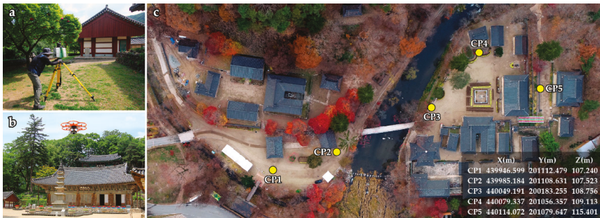
Figure 2. Equipment and methods used for 3D digital documentation: (a) terrestrial laser scanning using a specialized external camera; (b) hexacopter unmanned aerial vehicle (UAV); (c) five ground control points.
