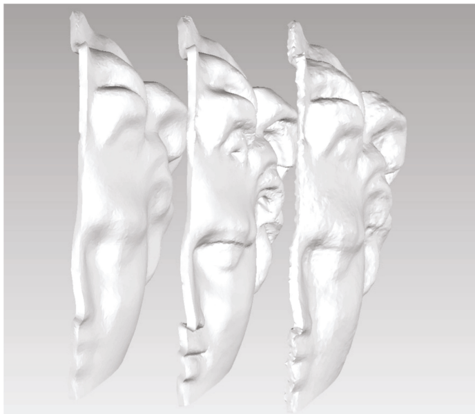
Figure 12. The three digital models: from the left: the first photogrammetric model, the laser-scanning model, and the second photogrammetric model.
