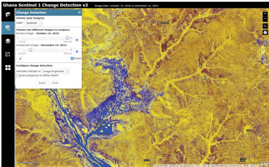
Figure 8. Change detection web application showing Sentinel 1 radar data of the Volta River area in central Ghana. The RGB is created as VV, VH, VV/VH. This application was created with the Change Detection web application template.
