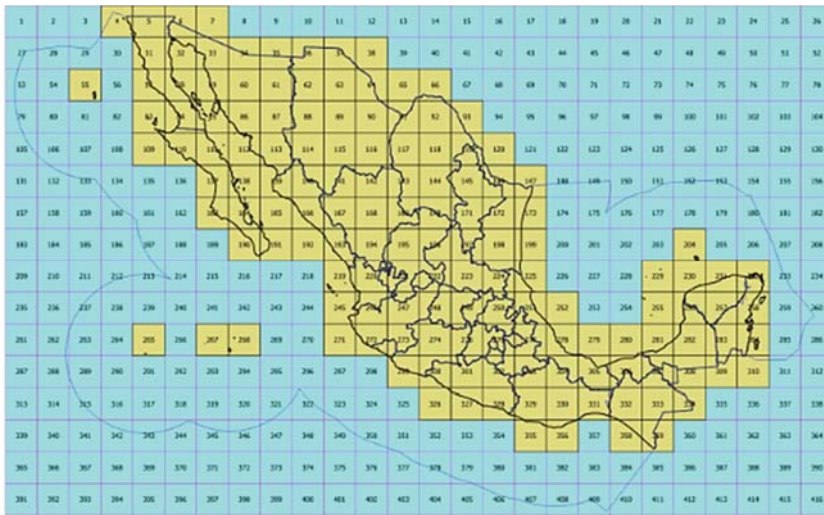
Figure 5. Overview of the standardized grid that is used for the MGDC (each tile represents a 150 × 150 km region).
