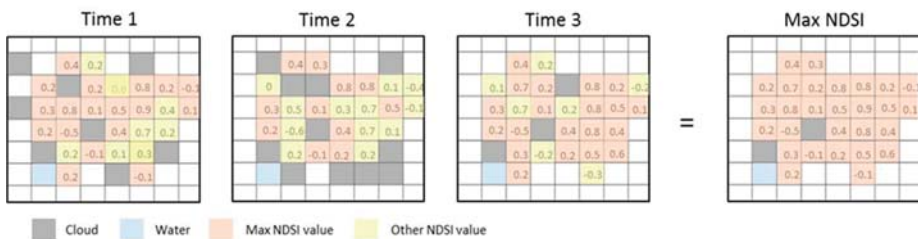
Figure 4. An example of the mosaicking technique employed to derive the maximum normalized difference snow index (NDSI) for a given month. From the available images (three in this example), NDSI was derived and the highest NDSI value was retained for the NDSI threshold test.
