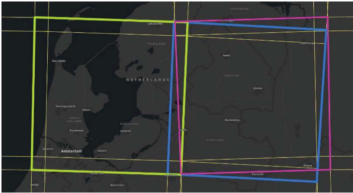
Figure 2. Sentinel 2 tile boundaries as thin yellow lines, with three highlighted tiles overlapping in central Netherlands. The green tile is predominantly in UTM zone 31, and the blue and magenta tiles are predominantly in UTM zone 32.
