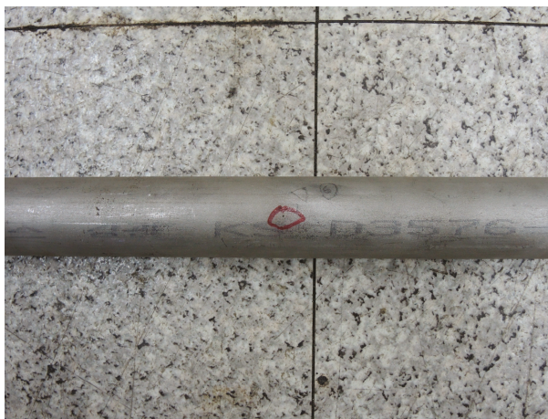
Figure 6. A simulated leak orifice of the pipe.
