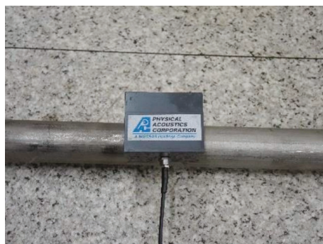
Figure 7. The AE sensor mounted with the magnetic hold down and vacuum grease couplant.
