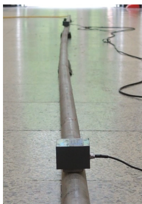
Figure 9. The placement of two AE sensors along the pipe.
