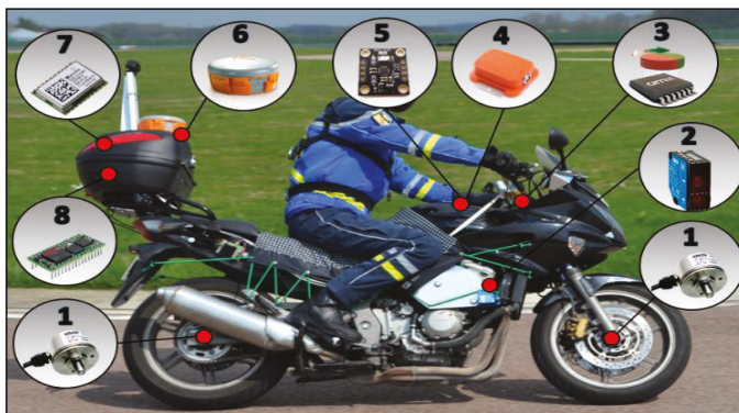
Figure 1. The ANR team instrumented motorcycle.
