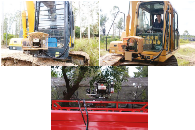
Figure 2. Measuring system installed at different forestry machines for operations experiment.
