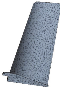
Figure 3. Finite element model of the blade.
