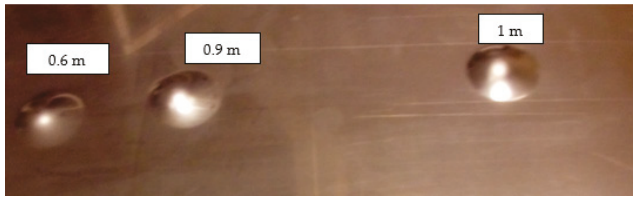
Figure 6. Tested metal sheet deformation after the impact of 1 kg weight from different heights: 0.6, 0.9, and 1.0 m.
