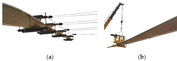
Figure 3. Full-scale static experiments of the wind turbine blade. (a) Side pulling in the full-scale static experiment of the wind turbine blade; (b) Lifting in the full-scale static experiment of the wind turbine blade.
