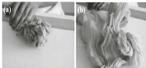
Figure 14. The Ni-Ti embedded fabric (a) crushed and (b) self-recovered “Reproduced with permission from [48], IOS Press, 2004”.
