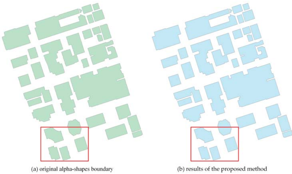
Figure 11. Visual comparison of the 2D building footprint generalization in Area-5. (a) original alpha-shapes boundary; (b) results of the proposed method.
