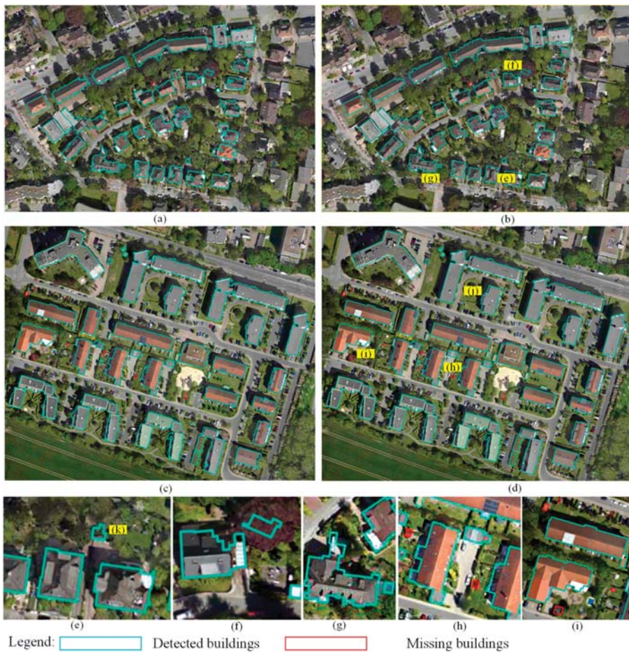
Figure 19. (a,b) Building detection and regularization on LN 2; (c,d) Building detection and regularization on LN 3; (e–g) Building regularization example in LN 2; and (g–i) Building regularization examples in LN 3.
