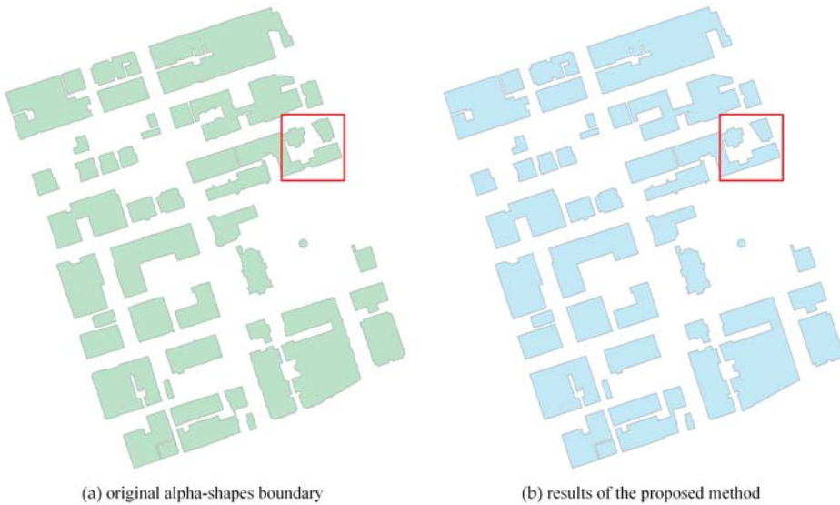
Figure 10. Visual comparison of the 2D building footprint generalization in Area-4. (a) original alpha-shapes boundary; (b) results of the proposed method.
