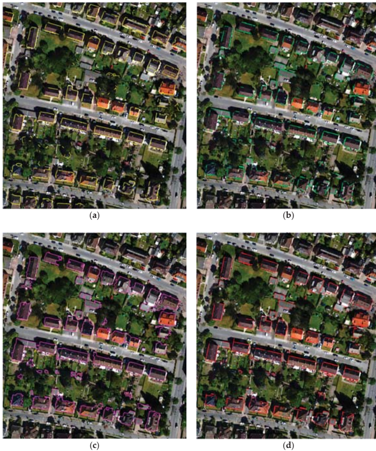
Figure 6. The extracted building edges: (a) the extracted building edges from DIM points; (b) the extracted building edges from orthophoto; (c) the extracted building edges from building blob; (d) the generated matched lines from original aerial images.
