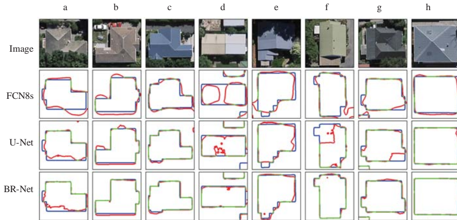
Figure 9. Representative results of single-building-level outline extraction by FCN8s, U-Net and, BR-Net. The green, red, blue, and white channels in the results represent true positive, false positive, false negative, and true negative predictions, respectively.
