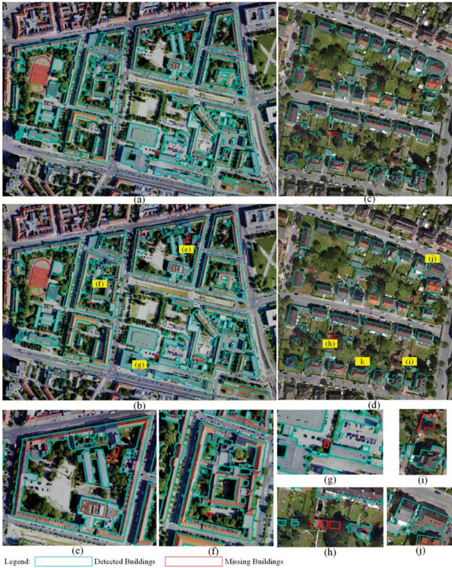
Figure 18. Building detection on the Potsdam and LN datasets: (a,b) building detection and regularization on the Potsdam dataset; (c,d) building detection and regularization on LN1; (e–g) building regularization example in Potsdam; (d,e) and (f–h) building regularization examples in LN1. Areas marked in (b) and (d) are magnified in (e–g) and (h–i), respectively.
