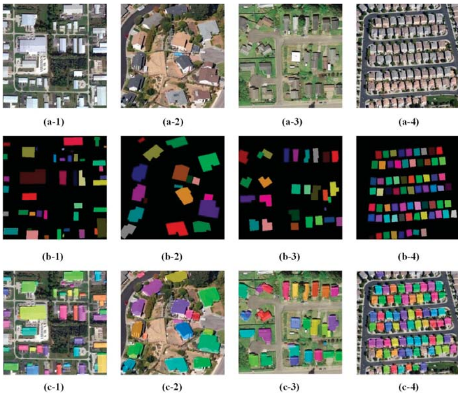
Figure 7. Examples of building recognition result for (a1–a4) original image. (b1–b4) Examples of test sample masks (color = positive; black = negative). (c1–c4) Building recognition result (color mask is recognition mark).
