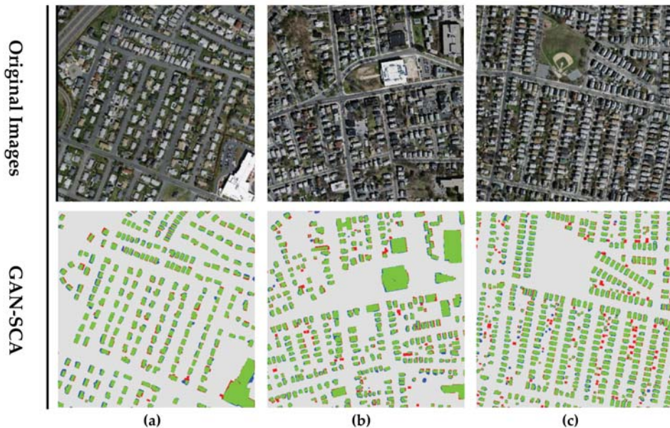
Figure 7. Building extraction results on the Massachusetts buildings dataset. (a–c) prediction results of three image patches in Massachusetts buildings dataset. Green: true positive (tp) pixels; Gray: true negative (tn) pixels; Blue: false positive (fp) pixels; Red: false negative (fn) pixels.
