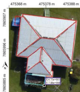
Figure 9. Extracting X and Y coordinates of a point of the cyan plane, where X and Y values are highlighted by a purple box.
