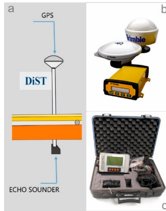
Figure 5. (a) Installation positions of the GPS and echo sounder on drone; (b) Trimble DSM232 GPS; (c) Omex Sonarlite echo sounder.
