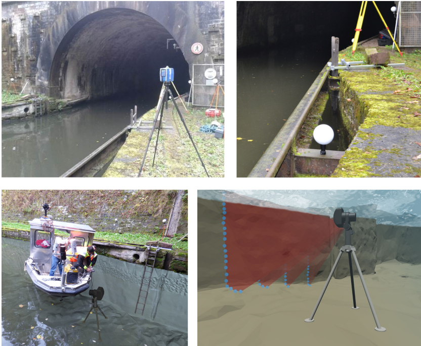
Figure 5. Data acquisitions in Niderviller’s tunnel: Photograph of the TLS device ( Top-left ); Zoom on a spherical targets and a ladder fixation on the dock side ( Top-right ); Schematic representation of MSS device positioning ( Bottom-left ) and Rotary scanning ( Bottom-right ).
