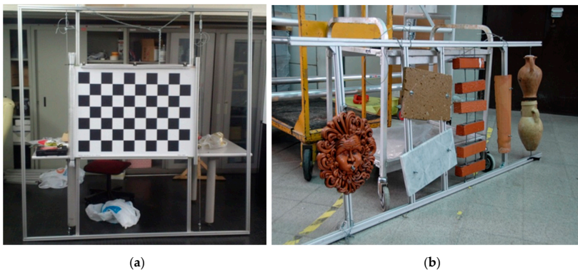
Figure 6. Orientation fixture (a). Target made of objects with different materials and shapes (b).
