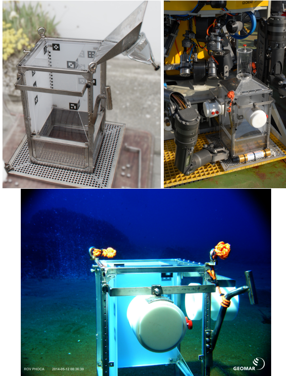
Figure 2. Three views of the bubble box, from left to right : box without cameras during development, box on ROV Phoca before being deployed (research cruise on RV Poseidon) and box in shallow water near Panarea, an area with heavy carbon dioxide release.
