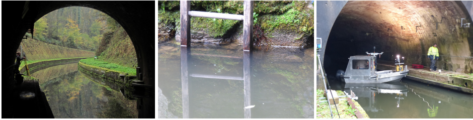
Figure 2. Constraints that apply to recording systems in tunnel canals. (Left) Global navigation data are not available in tunnels, nor at their entrances, because satellites are masked, hindering conventional mobile mapping; (Center) The turbidity of water prevents using optical imaging devices; (Right) The canal is shallow and narrow, so robust sonar processing algorithms are needed.
