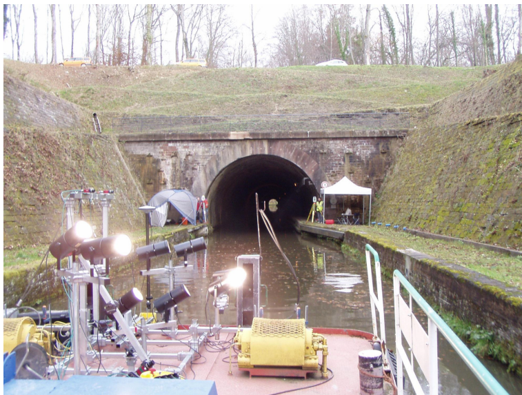
Figure 1. Modular on-board mobile image recording system at the experimental site.
