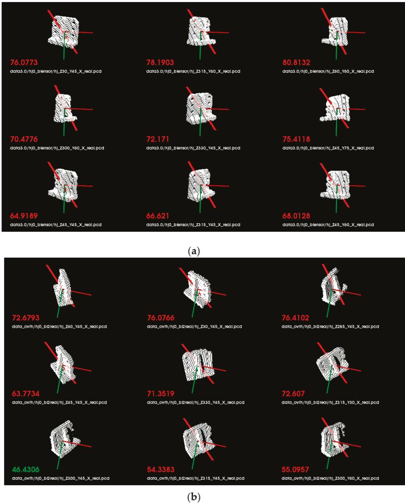
Figure 18. Matching results for (a) VFH descriptor and (b) OVFH descriptor.
