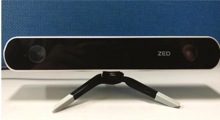
**Figure 11.** ZED stereo camera used in this experiment.
