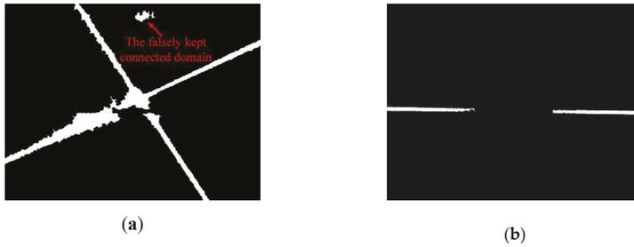
**Figure 7.** Kept connected domains. (a) Laser stripe region. (b) Joint region.
