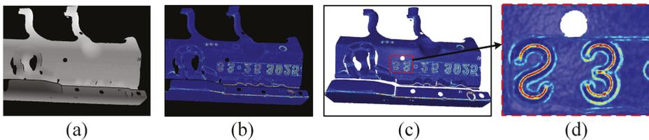
**Figure 2.** (a) A depth map acquired with the FPP sensor, (b) Its corresponding curvature map estimated using our method, (c) The rendered 3D point cloud with its color mapped from the curvature map, (d) Local details of curvature information at local point cloud surface.
