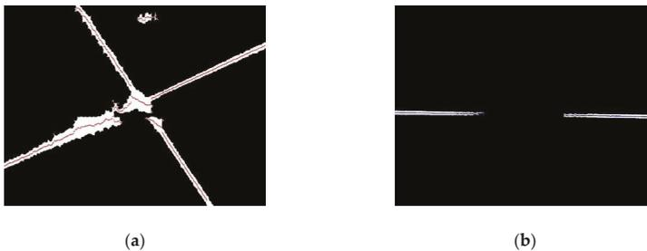
**Figure 8.** Extracted valid points. (a) Laser stripe region. (b) Joint region.
