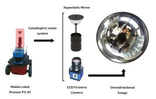
**Figure 1.** Real equipment constituted by a Pioneer P3-AT robot equipped with an internal odometer, a SICK-LMS200 laser range finder, and a catadioptric vision system, namely an omnidirectional vision system. This vision system is composed of a CCD (Charge-Coupled Device) FireWire DMK21BF04 camera, assembled with a hyperbolic Eizo h Wide 70 Mirror.
