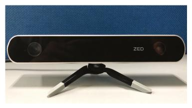
Figure 11. ZED stereo camera used in this experiment.
