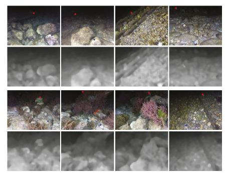
**Figure 6.** Examples of underwater images taken with our system and the computed rough depth using only the luminance channel. The rough depth was used later to speed up the stereo matching procedure. The red dots show the minimum detectable disparity ( $\approx$ 130 pixels in 10 cm baseline setup), while the blue dots show the maximum disparity ( $\approx$ 450 pixels in 10 cm baseline setup). See Figure 3 for corresponding distances and conversion to other baselines.
