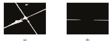
Figure 8. Extracted valid points. (a) Laser stripe region. (b) Joint region.
