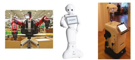
**Figure 9.** The three robot platforms used to evaluate the performance of our approach: the *Baxter* robot [33] (left), the *Pepper* robot [34] (center) and the *Hobbit* robot [35] (right).
