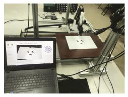
Figure 14. Automatic sorting system with machine vision.
