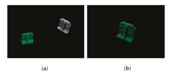
**Figure 11.** Registration results: (**a**) Initial relative pose; (**b**) Refined pose after the iterative closest point (ICP).
