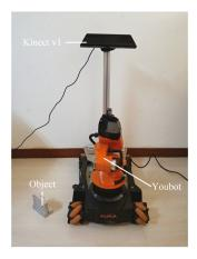
Figure 15. The hardware setup of the robotic grasping experiment.
