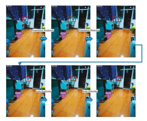
**Figure 3.** Visualization of the separate translation and scale prediction and detection on the video sequence of UAV. The previous position and scale are indicated by red bounding box, and the predicted position and scale are denoted in green, and the detected position and scale are shown with blue bounding box.
