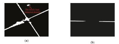
Figure 7. Kept connected domains. (a) Laser stripe region. (b) Joint region.
