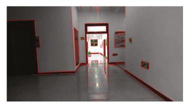
**Figure 3.** Common low-texture environment in an indoor scene with white walls, and point features (green x marks) extracted using ORB algorithm and line segment features (red lines) extracted using LSD algorithm.
