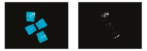
Figure 8. An image taken with no red component in illumination (illumination RGB were set to 0, 225, and 255, respectively), and its R-channel image.
