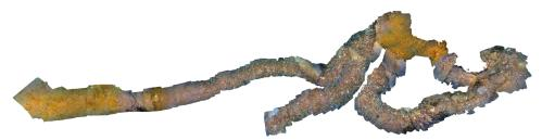
**Figure 14.** An example of the long trajectory 3D reconstructed model using images captured with the ROV-attached system. Such trajectories were used as ground truths to validate and tune the proposed method.
