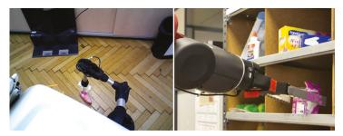
**Figure 4.** *Tricky* RGB situations of non-grasping contact points where a visual alignment between an object and the robotic manipulator can be confusing.
