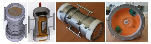
Figure 1. The handheld stereo system design and prototype.
