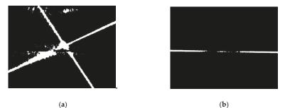
Figure 6. ROI after close operation. (a) Laser stripe region. (b) Joint region.
