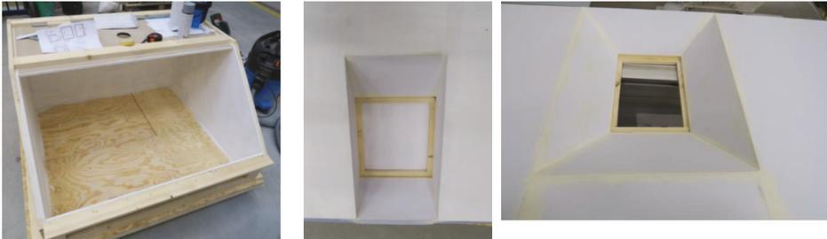
Figure 8. Model of a room for daylight measurement with changeable pitched roof.
