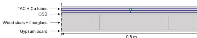
Figure 6. Simplified 2D COMSOL model used for annual simulation with symmetric boundary conditions at the two edges.
