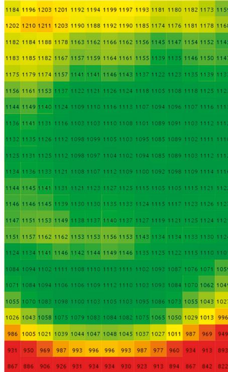
**Figure 13.** Distribution of solar radiation intensity on the surface comprising the tested samples. Location of lamps perpendicular to the tested samples. Minimum intensity 822W/m<sup>2</sup>, maximum 1211 W/m<sup>2</sup>, medium 1104 W/m<sup>2</sup>.
