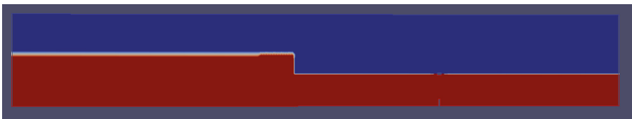
Figure 3. For the dam-break approach, the simulation domain is elongated and a water volume is placed on top of the initially still water surface.
