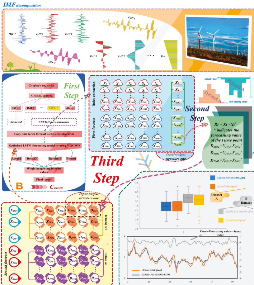
Figure 1. Explicit processes of data input and complementary ensemble empirical mode decomposition (CEEMD) parts of the CEEMD-fuzzy time series (FTS) multi-objective grey wolf optimizer (MOGWO)-LSTM (CFML) model.
