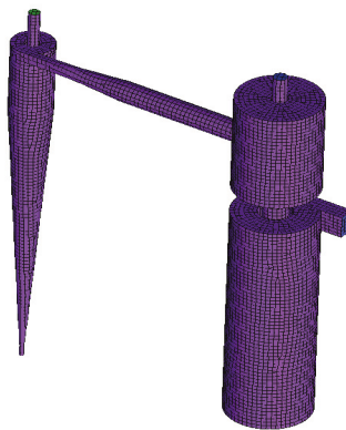
Figure 7. The meshing of four-products hydrocyclone.
