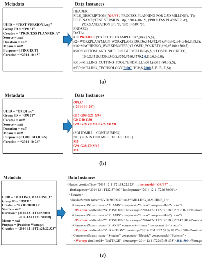
Figure 5. Data retrieval using a metadata-based search (a) ISO14649 program; (b) Numerical Control (NC) program; (c) MTConnect document. UUID: Universally Unique Identifier.
