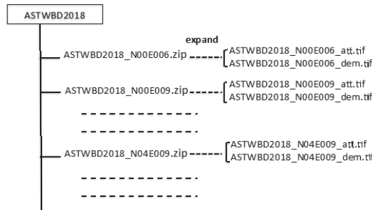
Figure 1. Advanced Spaceborne Thermal Emission and Reflection radiometer (ASTER) global water database (GWBD) folder structure.
