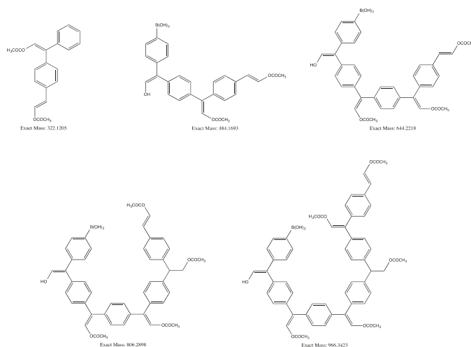
Figure 18. Proposed oligomer structures corresponding to HR-TOF MS data. From top left, n = 2, 3, 4, 5, and 6 where n = number of monomer units in the oligomer.
