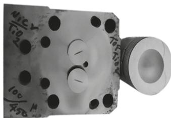
**Figure 20.** Photographic view of 450 lm TiO<sub>2</sub> coated piston, valves, and cylinder head (Reproduced from [59], with the permission of AIP Publishing).
