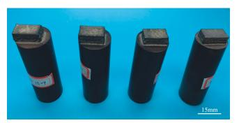
Figure 3. Macroscopic photograph of the W<sub>x</sub>NbMoTa alloys.
