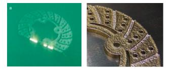
Figure 3. (a) Development of brake disc in EOS M-290 and (b) Disc brake developed by DMLS.
