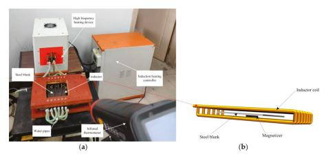
Figure 1. Localized induction heating system. (a) Experimental setup; and (b) schematic diagram of localized induction heating model.
