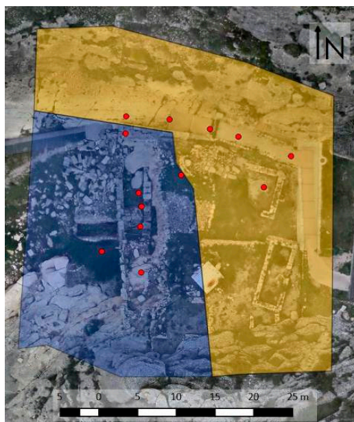
Figure 4. TLS stations distribution (red circles), including the area surveyed with TLS during the different campaigns performed (first campaign in orange colour and second campaign in blue colour).
