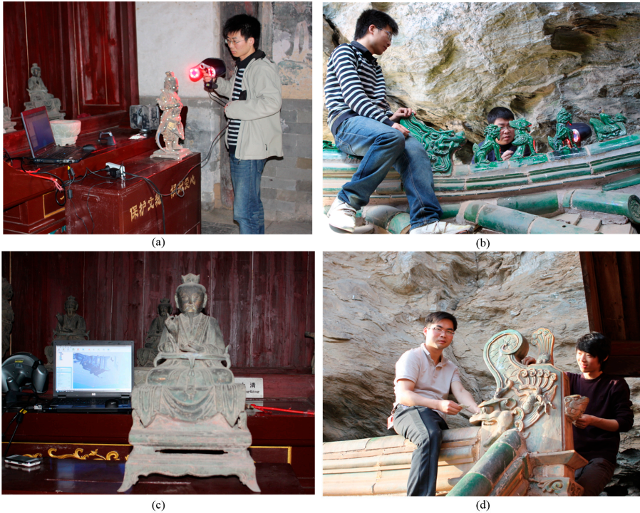
Figure 7. 3D data collection for some components with the handheld scanner. (a) Small statue scanning; (b) rows of horned beast scanning; (c) large statue scanning; (d) corner horned beast scanning.
