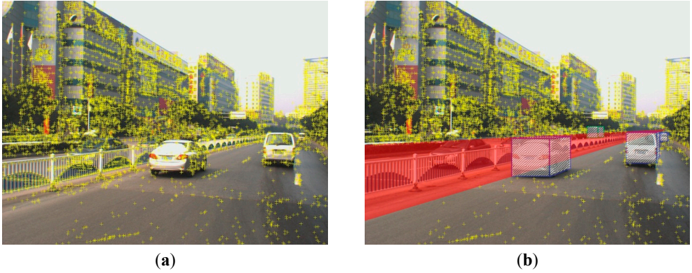
Figure 9. SIFT feature points removing results. (a) Original SIFT feature points set on image. (b) Mask results, which show the masked out features on the vehicle and guardrail regions.
