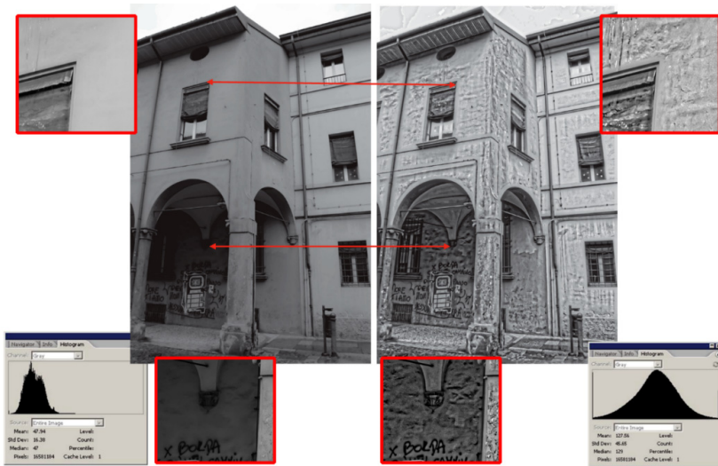
Figure 9. Example of the Wallis filtering procedure: note the much smoother and Gaussian-like histogram.
