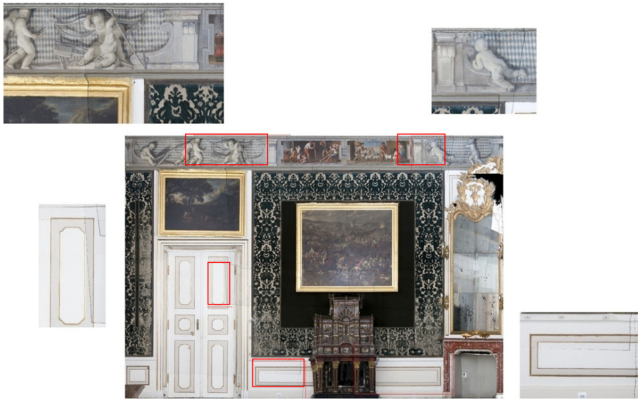
Figure 24. RGB orthoimage with marked overlaps and seam lines.
