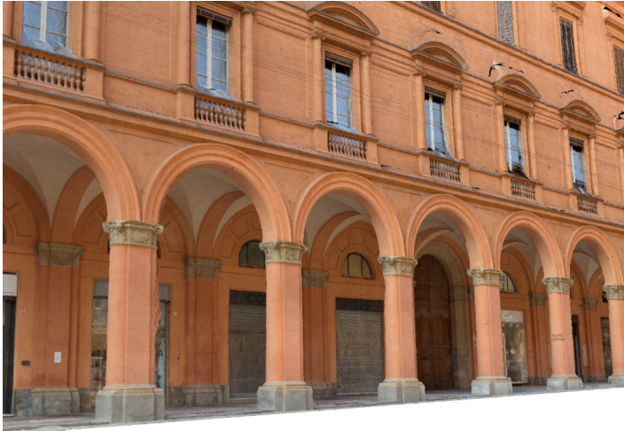
Figure 14. Example of dense 3D point cloud of a portico obtained with the presented photogrammetric methodology based on an advanced pre-processing pipeline.
