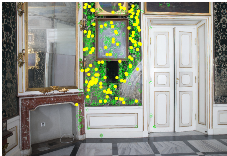
Figure 22. Example of utilized image with points used for orientation (control points, in green) and yellow “o”—check points.
