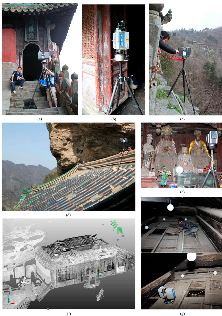
Figure 6. 3D data collection for the building. (a) Scanning for the gate; (b) scanning for the corridor; (c) scanning for the Longtou Incense; (d) scanning for the roof; (e) scanning for the statues; (f) point cloud of the whole building; (g) scanning for the attic.
