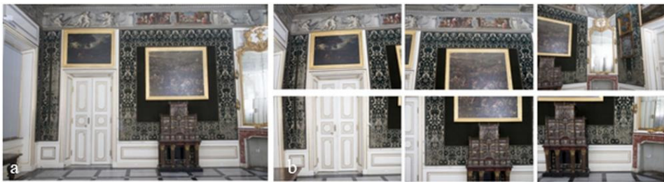
Figure 16. Examples of used images: (a) Variant I: one image covering the entire orthoimage area; (b) Variant II: part of multiple images covering the entire orthoimage area.
