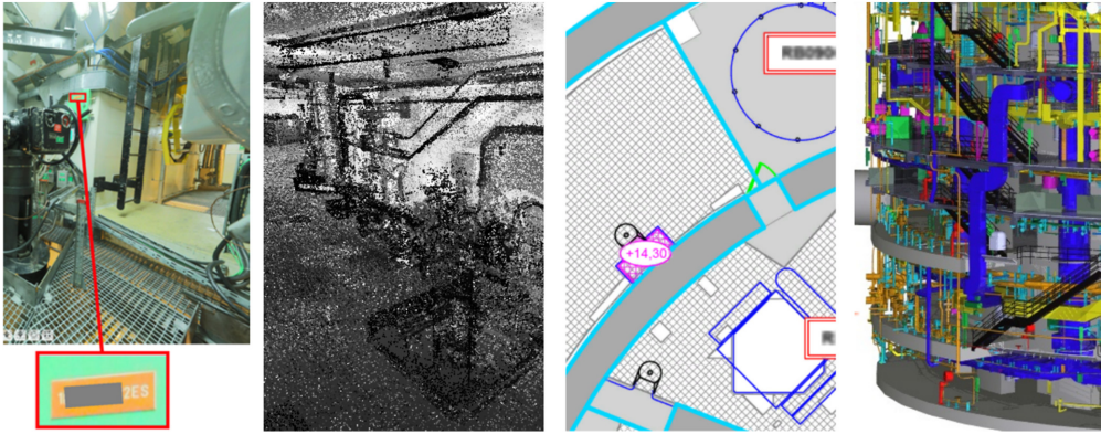
Figure 4. Four types of data are required to represent a power plant facility with a high degree of confidence (geometry and appearance): panoramic images, laser scans, floor maps and 3D CAD model.
