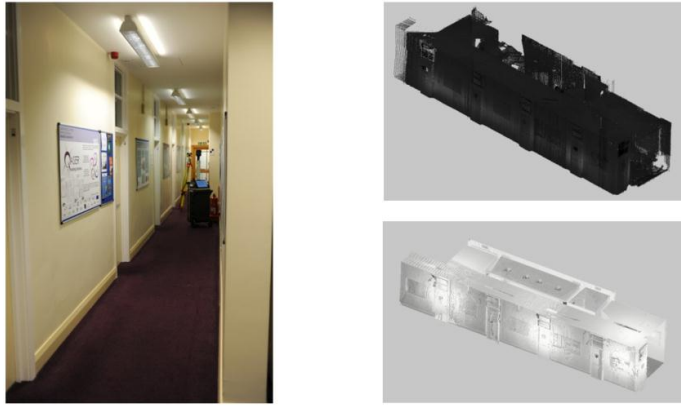
Figure 5. Image of corridor ( left ) and resulting point cloud data collected with a Viametris Indoor Mobile Mapping System ( top right ) and Faro Focus 3D S ( bottom right ).
