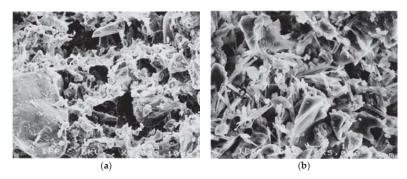
Figure 14. Morphology of cement particle under SEM (a) at 20 °C; (b) at 60 °C [19].
