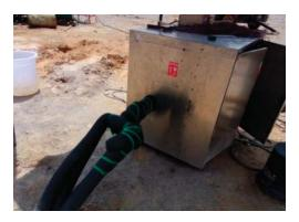
Figure 4. Thermal response tester.
