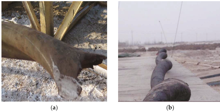
Figure 1. Tubing damage caused by perforating shock loads: (a) tubing breaking; (b) tube buckling.
