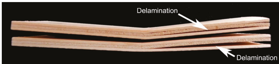
Figure 9. Delamination in the plywood samples prepared at 140 °C and 1 min during the determination of bending strength.
