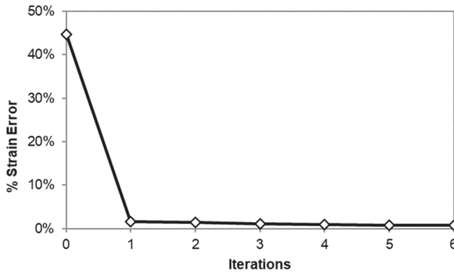
Figure 10. Weighted RMS strain error for the OHC FEMU methodology using FEM-generated virtual test strain data.
