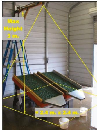
Figure 1. Illustration of rainfall simulator and test plots.
