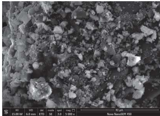
Figure 11. SEM photo of coal powder treated with SPI.
