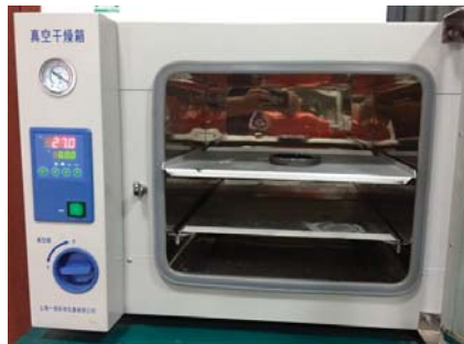
Figure 1. Vacuum drying chamber with a preset temperature.
