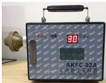
Figure 7. Coal mine dust sampler.
