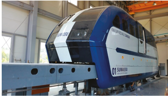
Figure 2. High-speed maglev based on the LSM.
