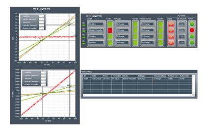
Figure 24. Test 2 (Closed-Loop): Total fault in HT2 ("Broken Propeller") with disabled fault accommodation.
