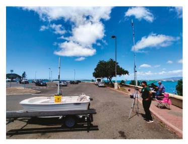
**Figure 2.** Over-land experimental setup. Ground station transmitting antenna (mounted on tripod, right), and trailered rigid tender serving as mobile station with receiving antenna (left).
