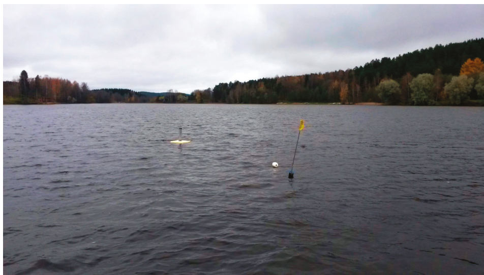
Figure 3. Online trap in Savilahti Bay basin at a depth of 6 m under the flag sign. Anchored float behind flag sign is the base station for the online trap, which sends measurements to the Internet over a mobile network.
