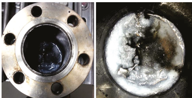
Figure 3. The sample pictures showing a massive wax formation in the reactor after an FTS reaction by carbon-supported catalysts that are evidently black with the wax being conspicuously white.
