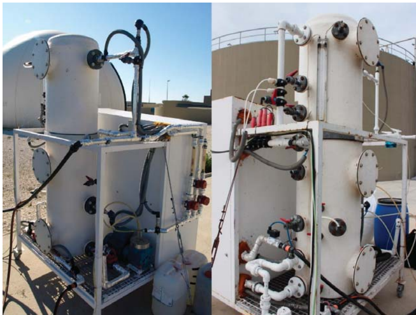
Figure 1. Photograph of the pilot scale anoxic biotrickling filter.
