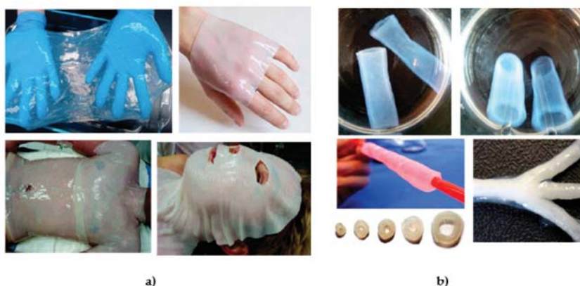
Figure 8. (a) BC dressings as produced and when applied on wounded torso, face and hand. Reproduced from [106], with permission from Biomacromolecules, 2007; (b) vascular graft and blood vessel tubes with different sizes and shape, produced by fermentation onto a branched silicone tube. Reproduced from [107–109], with permission from Frontiers, 2016, European Polymer Journal, 2014 and Biotechnology and Bioengineering, 2007, respectively.
