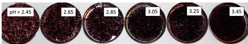
Figure 3. KHT precipitates from Concord juices as a function of pH.
