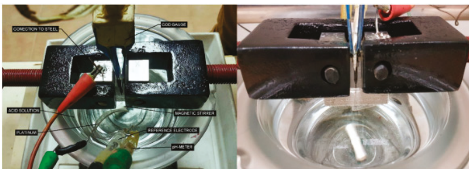
Figure 12. Set-up of the slow rate tests in environment using C(T) specimens.
