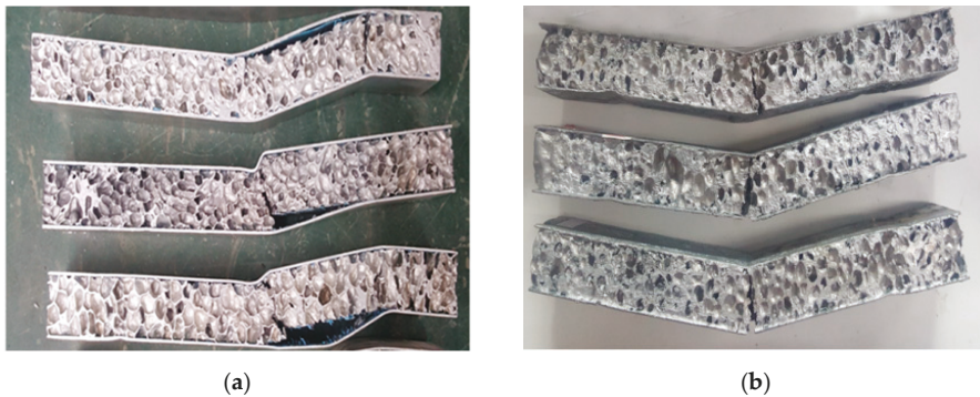
Figure 9. Fatigue fracture morphology of two types of AFS (a) adhesive joining samples (b) metallurgical joining samples.
