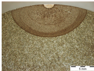
Figure 6. Representation of fracture surface for specimen utilized within Overload test #1.
