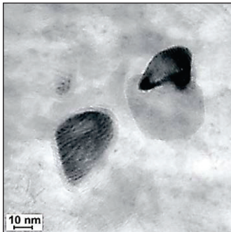
Figure 3. Precipitation of carbonitride (Ti,Nb)(C,N) with numerous small dispersive precipitates corresponding to the hardening of the steel. (a) recipitation of carbonitride (Ti,Nb)(C,N); (b) large particle-related EDX spectrum.
