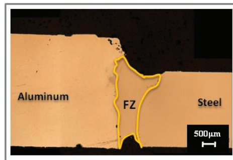
Figure 8. Optical macrograph of cross section obtained by LOW technique.
