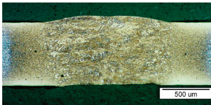
Figure 7. Overall photo of laser-welded steel HCT600X-HCT600X.
