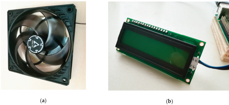
Figure 3. (a) Ventilation device used to simulate the controlled ventilation system in the prototyping box used (b) the LCD display screen used for development phases.
