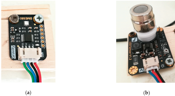
Figure 4. (a) the BME680 Temperature, Relative Humidity, Barometric pressure, and TVOC (Total Volatile Organic Compounds) gas sensor used; (b) the used Gravity Analog CO 2 gas sensor used.
